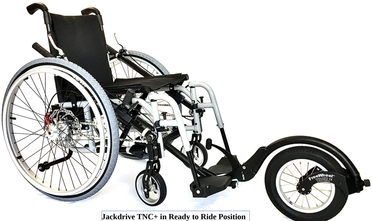
Rotate both Left and Right Pushrims in Opposite Directions to Maneuver The FreeWheel Backwards into The Riding Position
