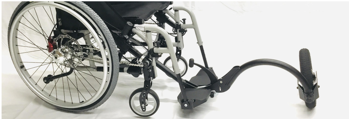
Rotate both Left and Right Pushrims in Opposite Directions to Maneuver The FreeWheel Backwards into The Riding Position
